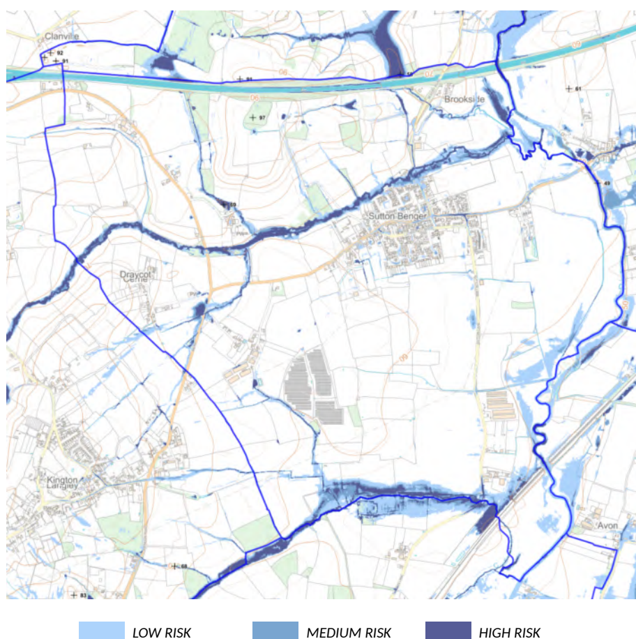
21. Map of flood Surface water flooding
